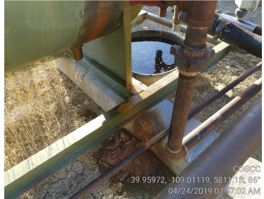
Photo 6. Open container with over flowing fluid and oily stained soil next to separator.
