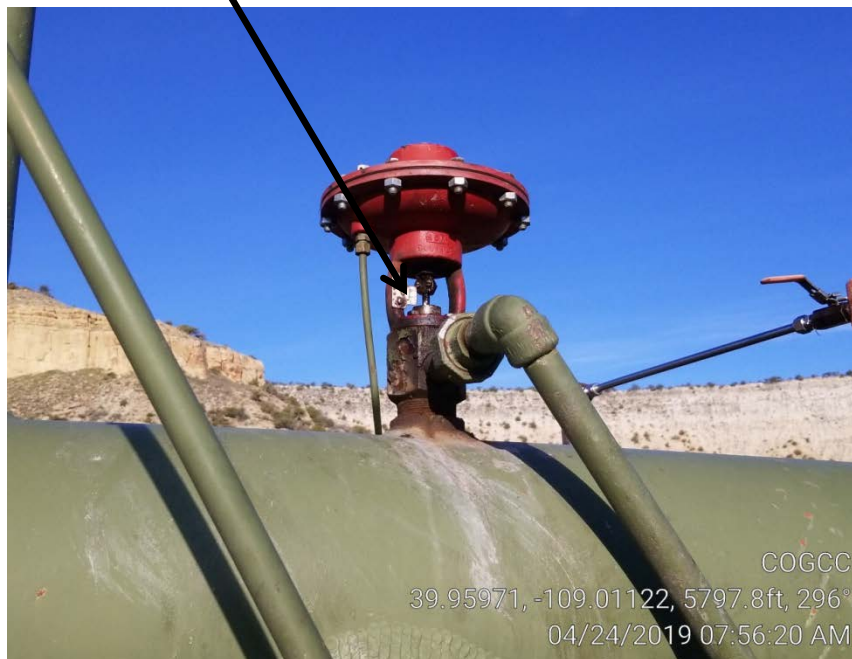
Photo 3. Gas leak on top of separator.
