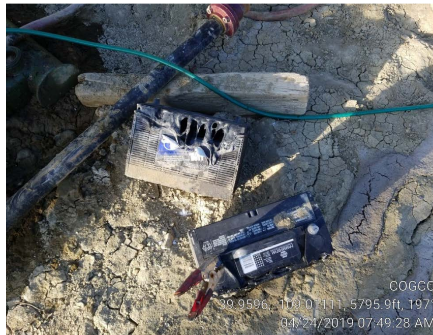
Photo 2. Partially melted lead batteries next to compressor.
