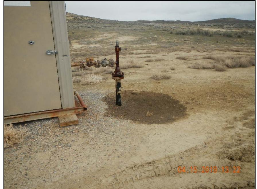
**Photo 2. Non reportable spill. Stained soil at meter run flowline.**
