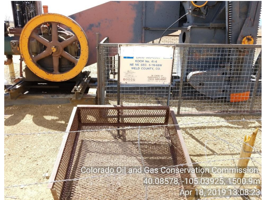
Photo 2 Location sign not legible and Unused equipment flywheel guard
