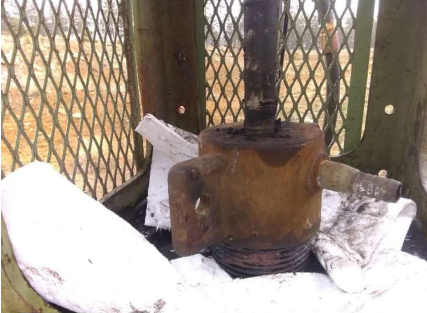
PHOTO 1: REPLACED THE PACKING TO ELIMINATE THE WATER LEAK. PACKINGS WERE SECURELY FASTENED. ABSORBENT PADS WERE USED TO DRY THE SURFACE, THEN REMOVED FROM LOCATION.
