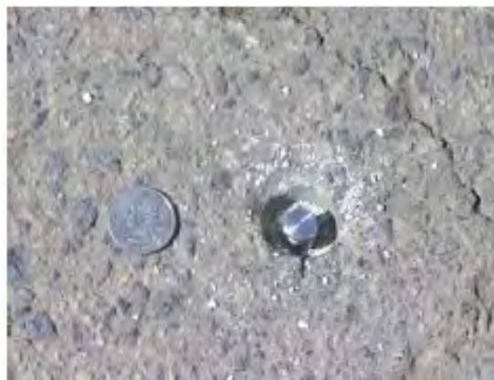
Example of flush mounted vapor sampling point
