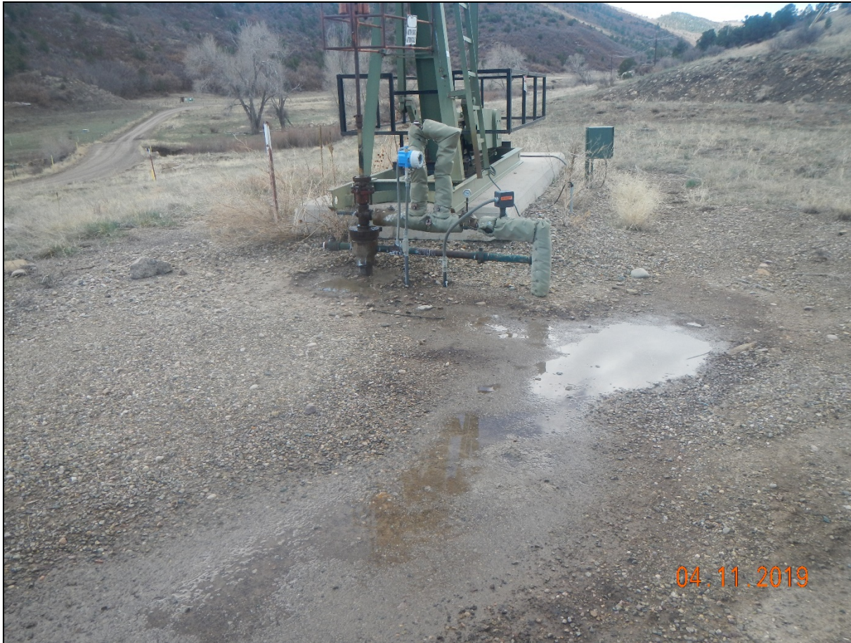
Photo 1. There is a dripping water leak from the wellhead.
