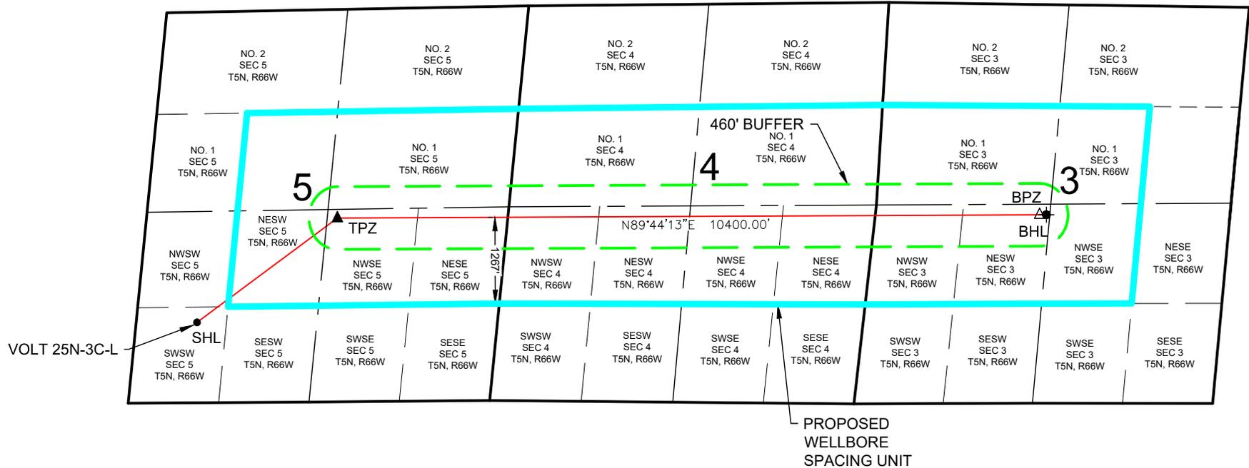
**VOLT 25N-3C-L WELL TO BE LOCATED 1178' FSL AND 888' FWL, SEC 5, T5N, R66W**
