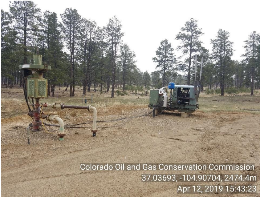
Photo 3 HR#32-15R WH and HYD motor skid
