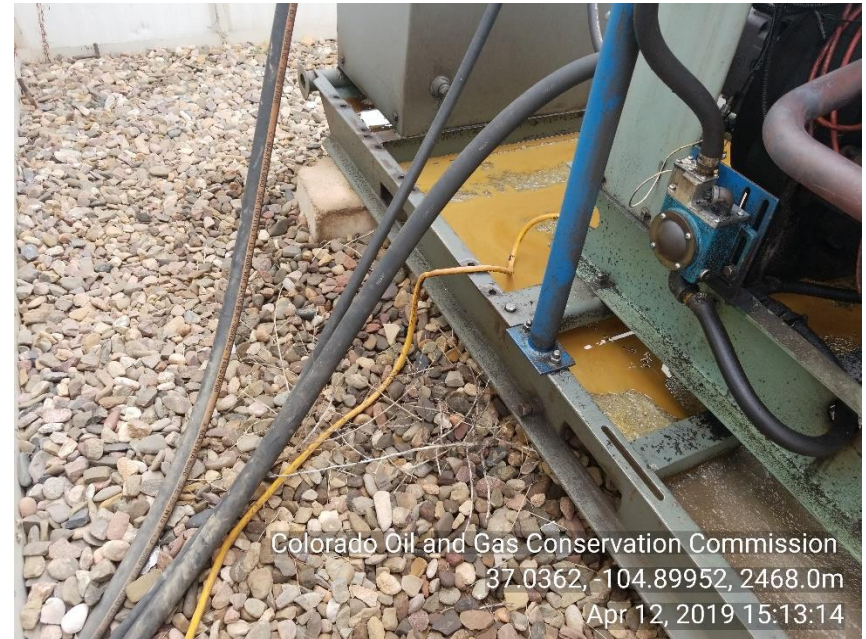
Photo 4 Stained soil around HYD motor skid
