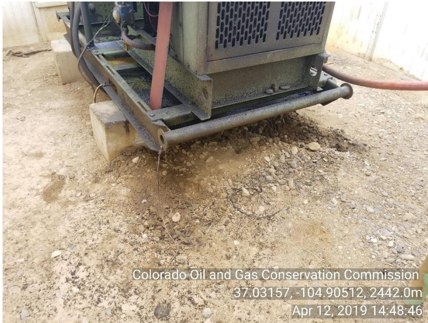
Photo 5 Stained soil; Around HYD motor skid
