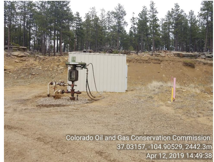
Photo 2 WH and HYD motor skid sound walls
