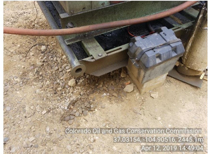
Photo 6 Stained soil around HYD motor skid
