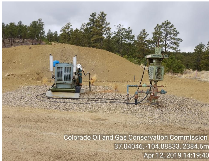
Photo 1 WH and HYD motor skid
