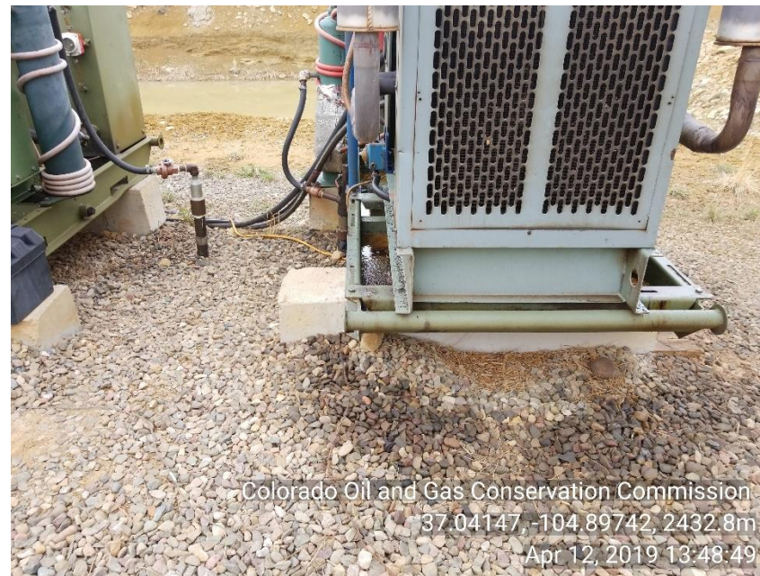
Photo 6 stained soil around both wells HYD motor skids
