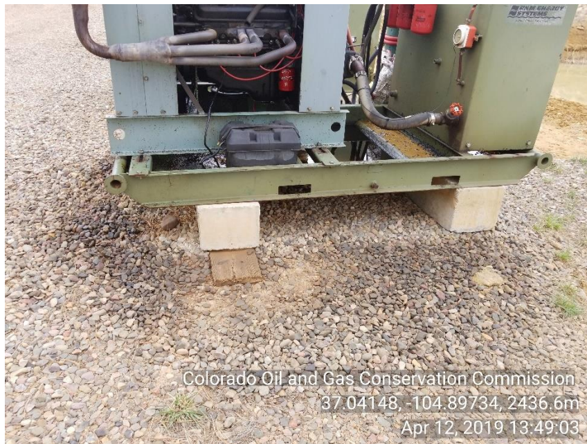
Photo 7 stained soil around both HYD motor skids.
