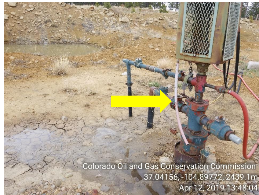
Photo 4 HR#33-06-02 Mechanical issue packing leaking and being drained through hose onto ground.
