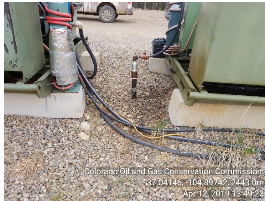
Photo 8 stained soil around both wells HYD motor skids
