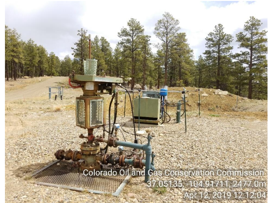
Photo 2 WH and HYD motor skid.
