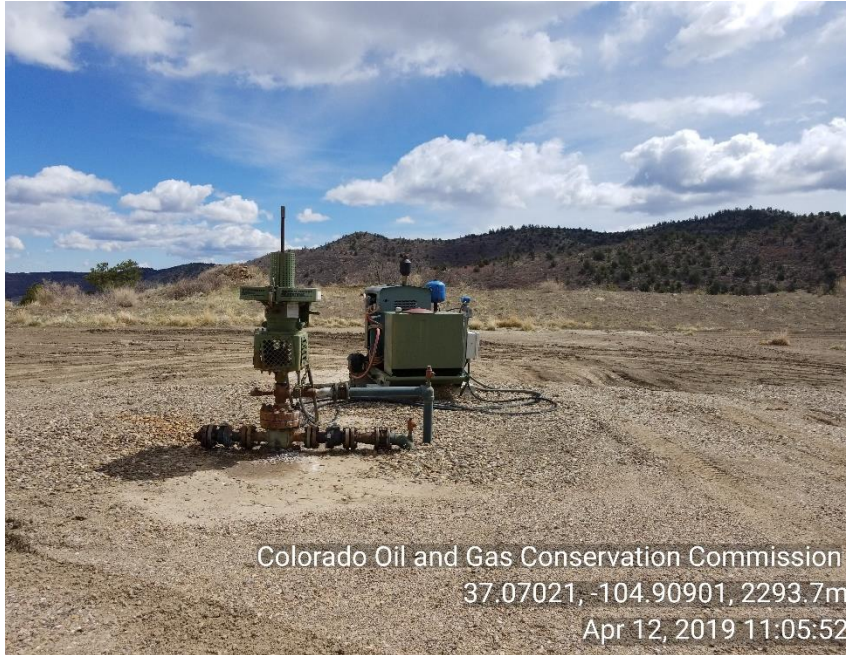
Photo 1 WH and HYD motor skid.
