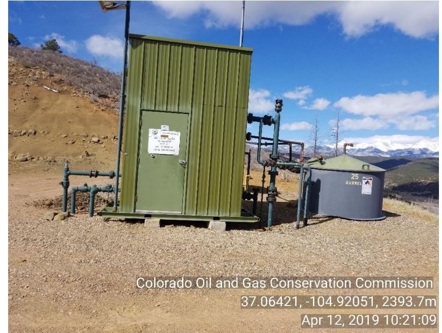
Photo 2 Sep/meter house and 25bbl produced water tank.
