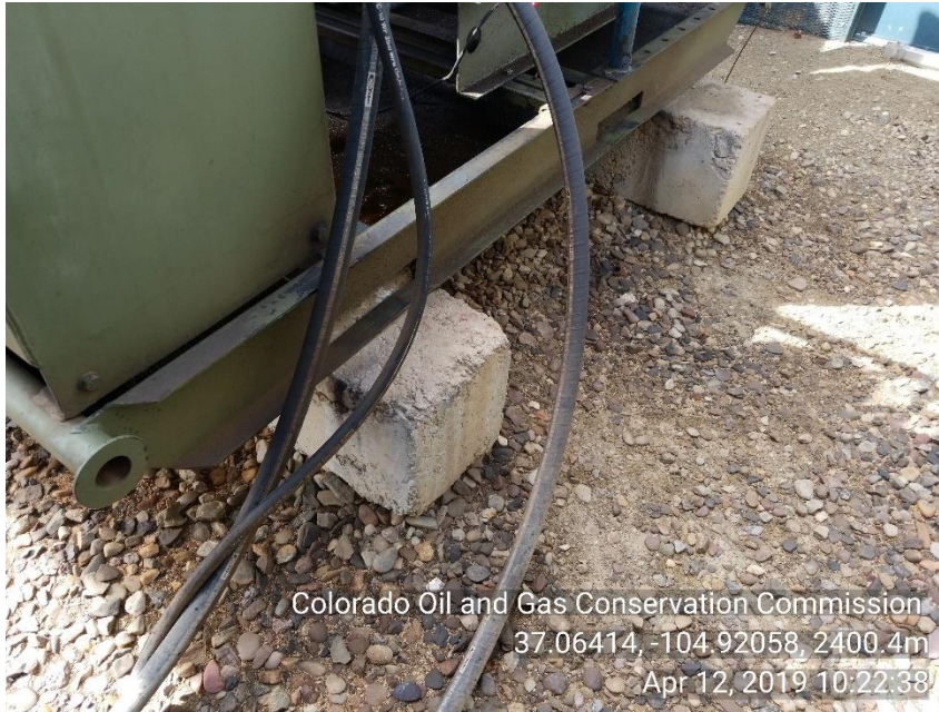
Photo 5 Stained soil around HYD motor skid.
