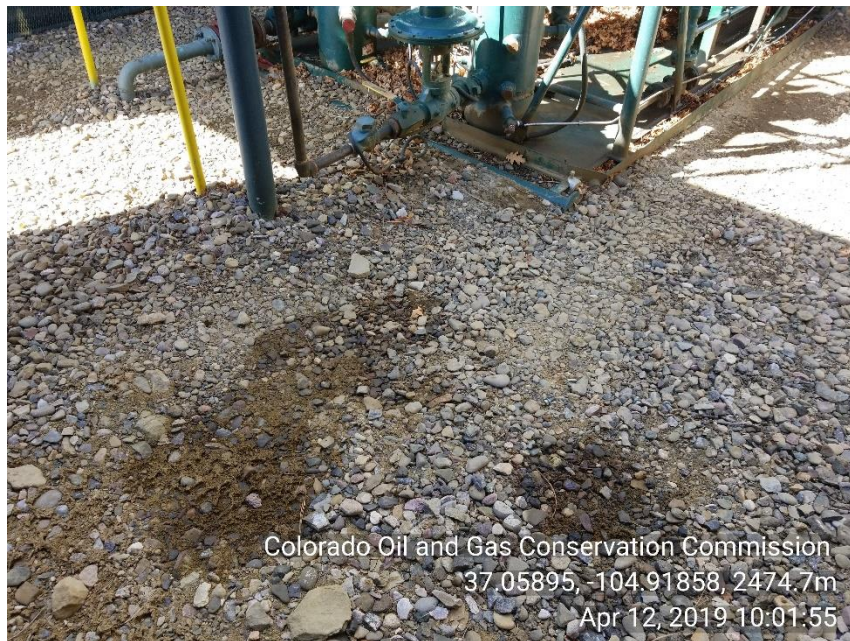
Photo 5 Stained soil around liquid ring skid.
