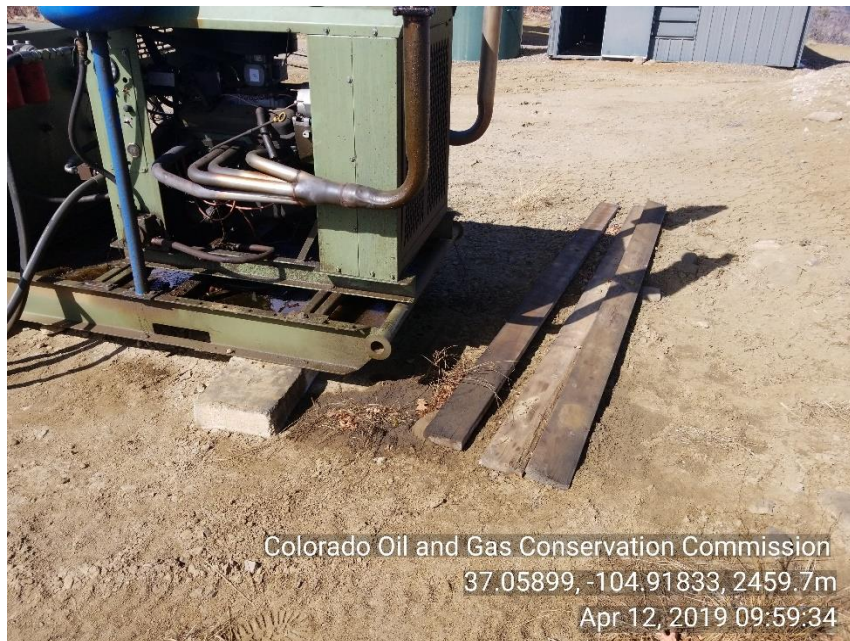
Photo 3 Stained soil around HYD motor skid. Trash (1x4 boards)
