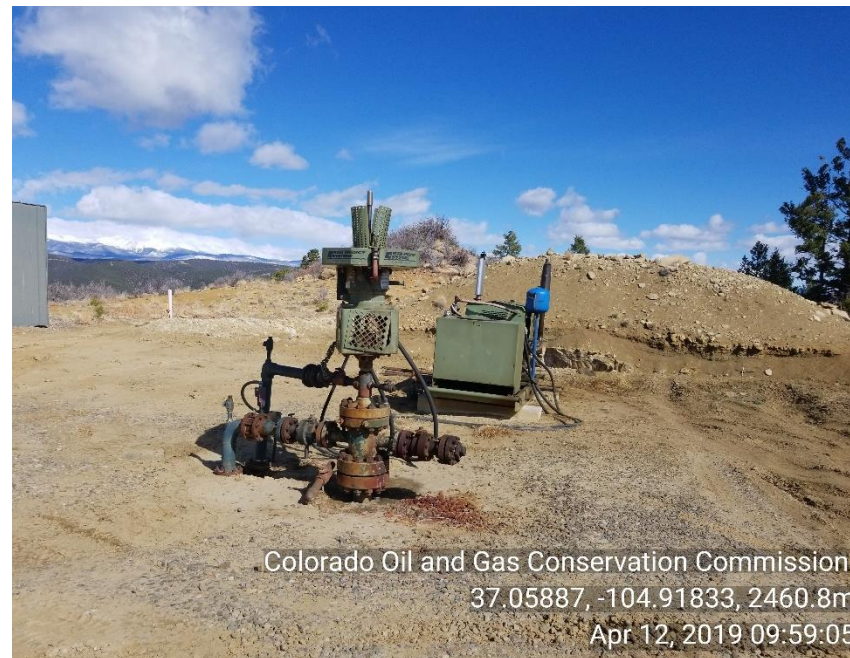
Photo 2 WH and HYD motor skid
