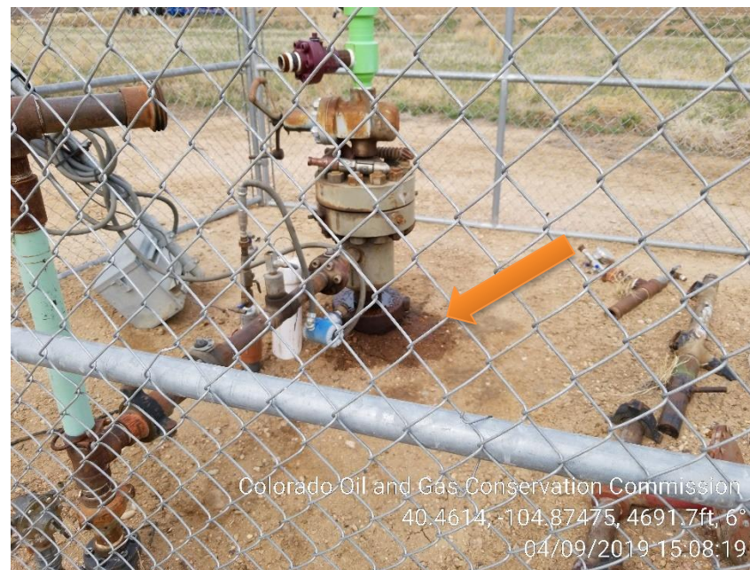
Photo 6 – Wellhead 27-51 Casing Collar leaking and stained soil
