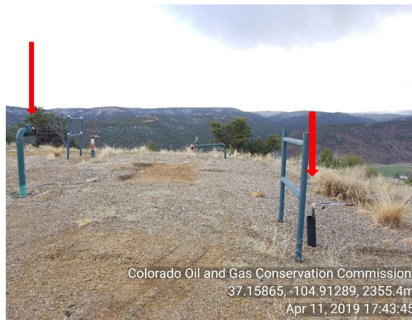
Photo 2 all production equipment removed. Unmarked, unused and LOTO risers
