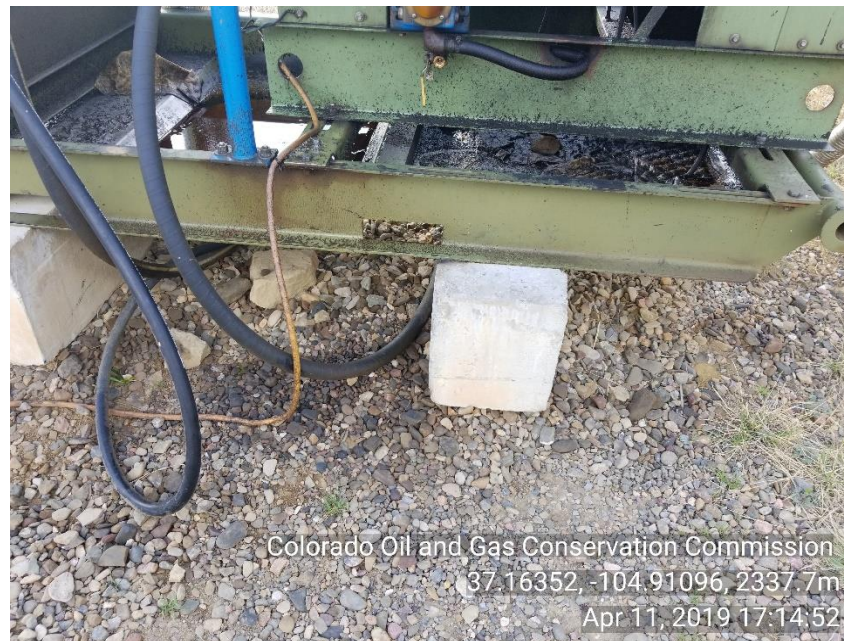
Photo 4 Stained soil around HYD motor skid
