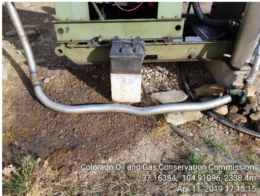
Photo 5 stained soil around HYD motor skid
