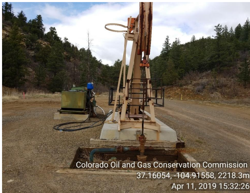
Photo 1 PU and HYD motor skid
