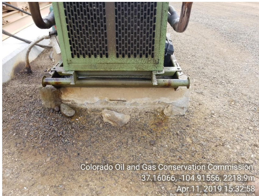
Photo 3 Stained soil around HYD skid
