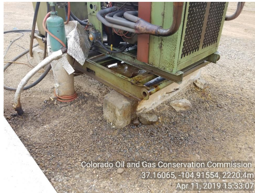
Photo 4 Stained soil around HYD skid
