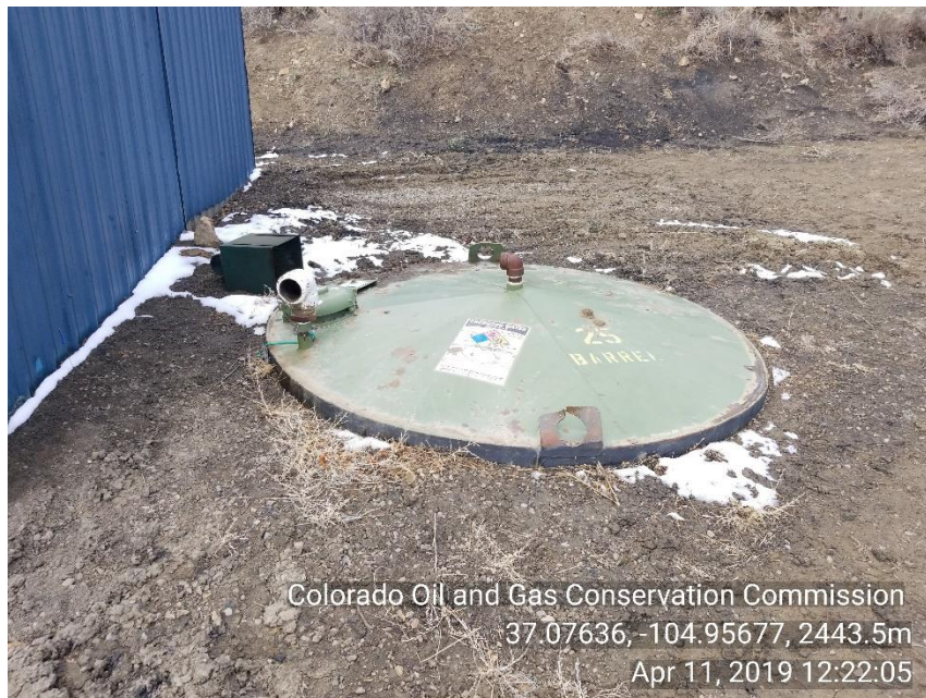
Photo 3 25bbl buried production tank. Wild life protection 2" 90's no bull plugs.
