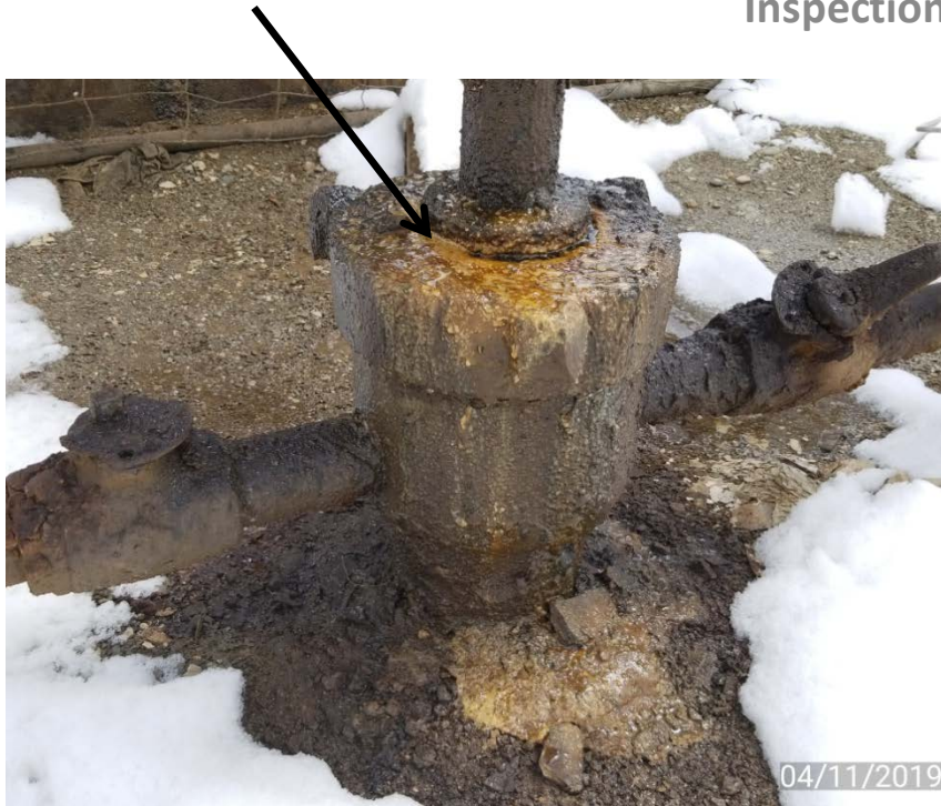
Photo 5. Well head leaking gas & oily waste on ground.
