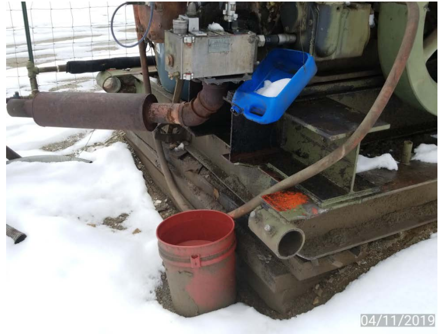
Photo6. Pump jack dripping lubricant into open bucket.
