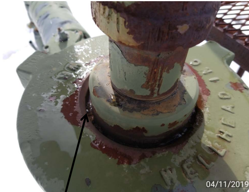
Photo 3. Gas leaking at well head.
