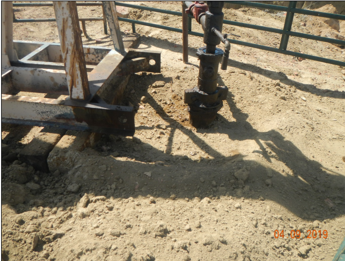
Photo 4. Oil stained soil still appears around the wellhead.
