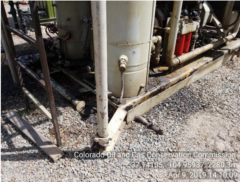
Photo 11 Stained soil around Liquid ring skid
