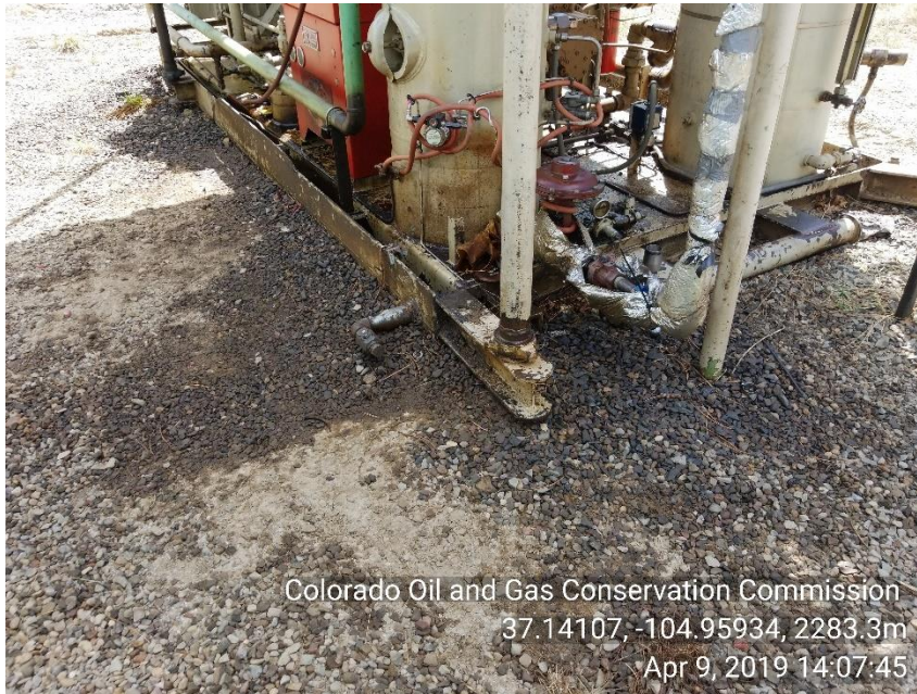
Photo 7 Stained soil around Liquid ring skid
