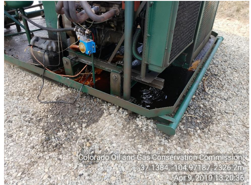
Photo 6 Stained soil around liquid ring skid
