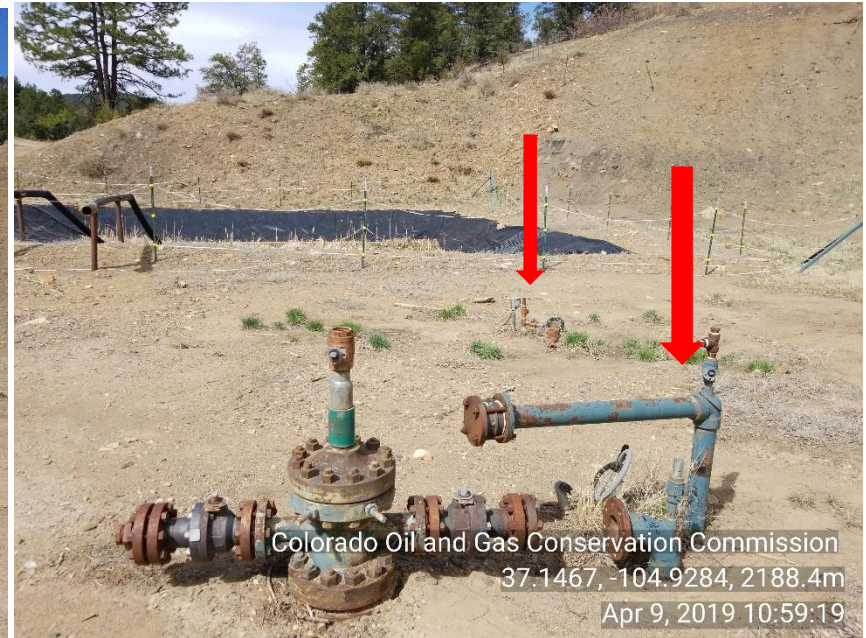
Photo 8 Unused equipment: unused unmarked not LOTO 2" piping and 1" electric lines
