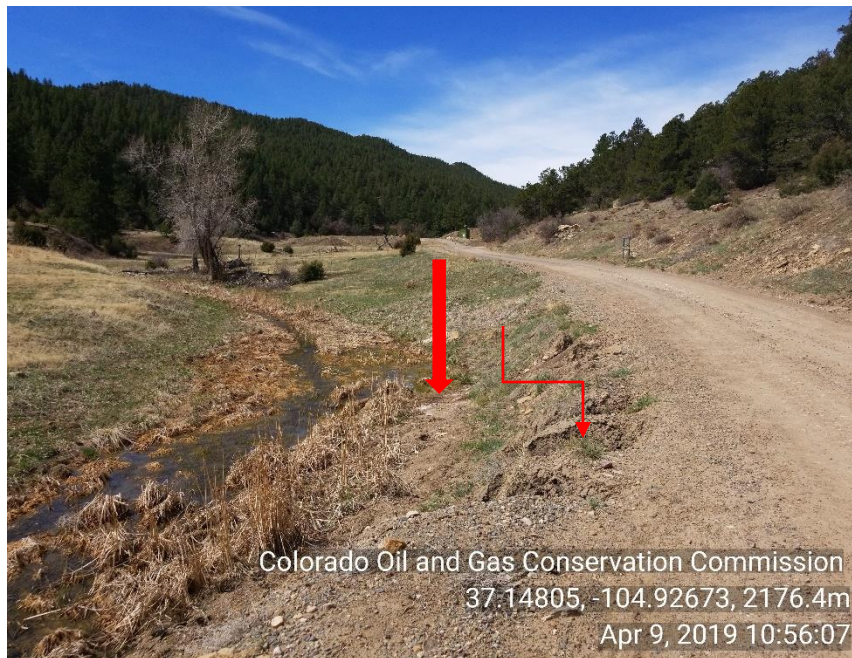
Photo 1 Storm water: Reels on road to location allowing sediment into water way
