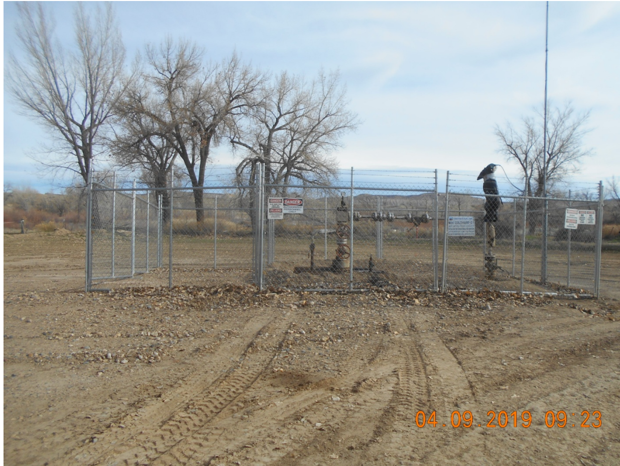
Injection Wellhead
