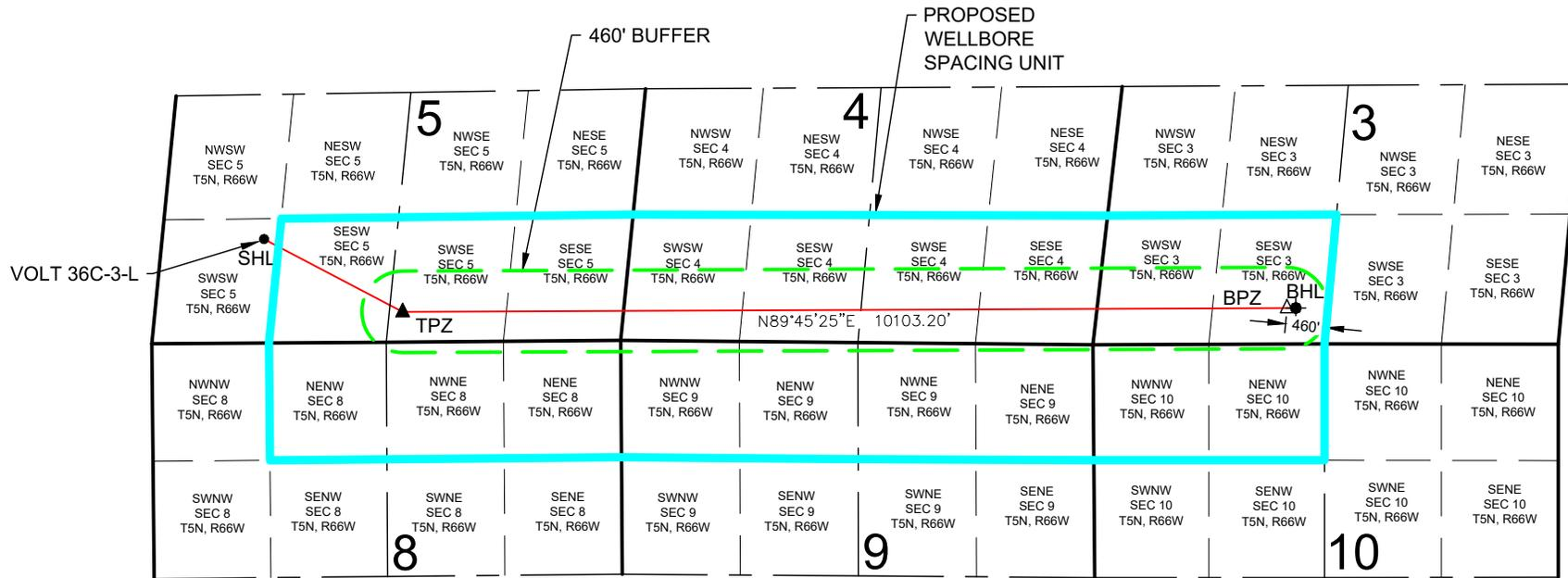
**VOLT 36C-3-L WELL TO BE LOCATED 1174' FSL AND 1147' FWL, SEC 5, T5N, R66W**
