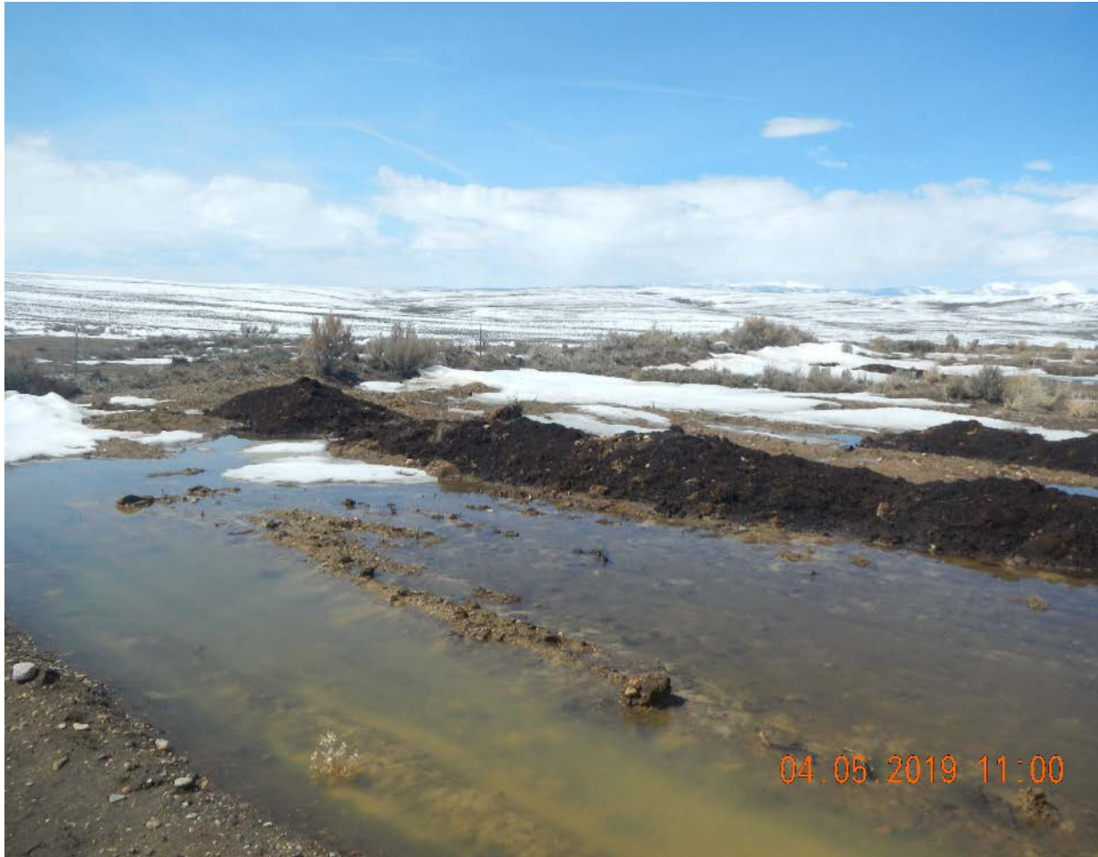
Photo 17 –Pooled water inside land treatment area. Some water had liquid hydrocarbon.
