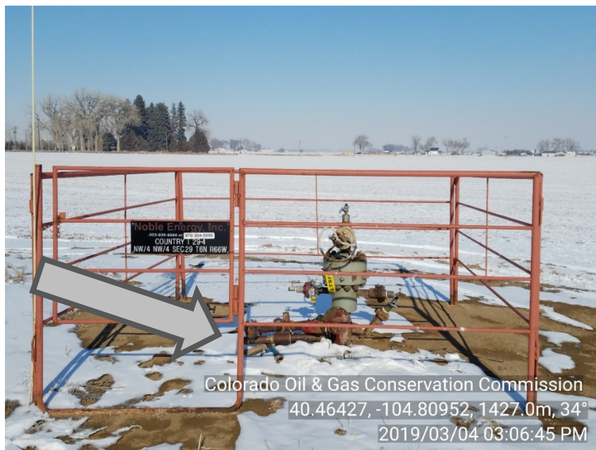
Photo #1 Country 1 29-4 (05-123-26421) Wellsite Temporarily Abandoned | TA Unused Equipment Orange Decommission tag NOT present from prior FIR
