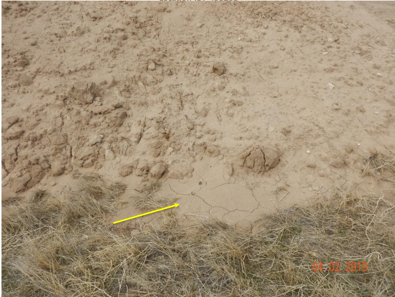
Photo 12: Photo taken from the soil stockpile. Photo show sediment deposition due to stormwater degradation and runoff from the soil stockpile.
