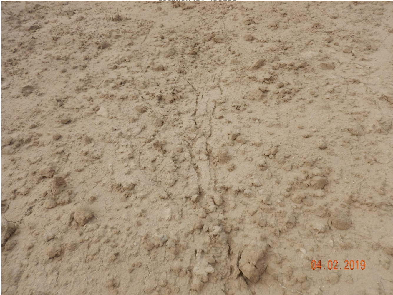
Photo 11: Photo taken from the soil stockpile. Photo shows erosion degradation evident on stockpile.
