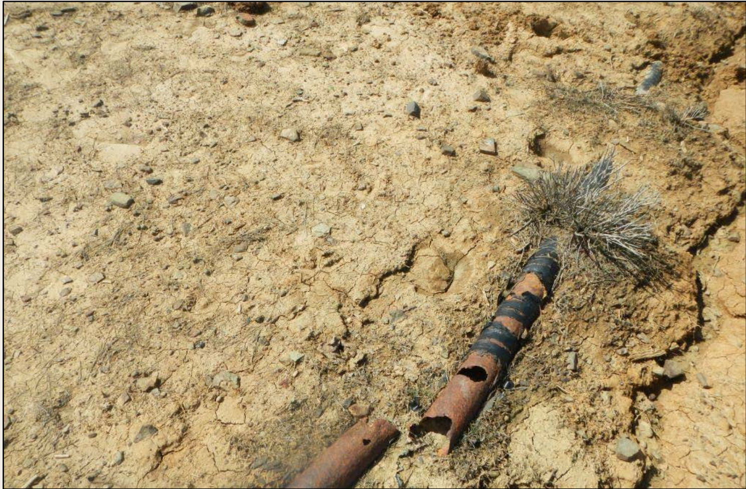
Photo 5. View of Corroded line that is no longer functioning.
