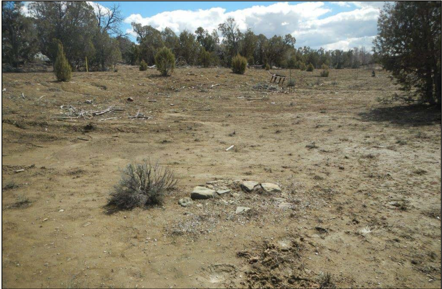
Photo 2. View of the eastern project area from the northern edge facing southward. Poor revegetation. Erosional run-on and sediment deposition observed, along with metal debris in background.
