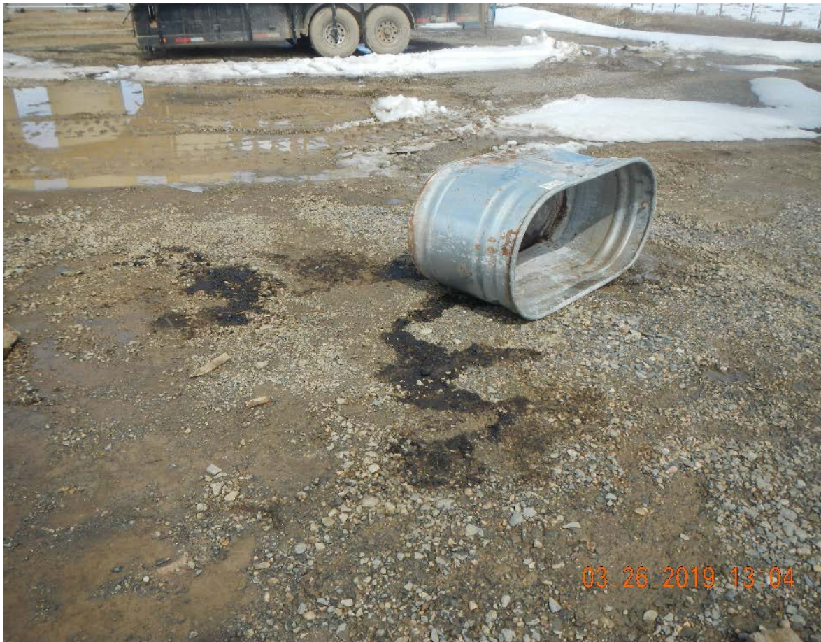
Photo 7- Overturned stock tank, stained soil. Spilled fluid and soil should be removed in 48 hrs (per COGCC Corrective Action matrix) and handled per COGCC rule 907. Note combustor in background. Photo is taken looking north, on the North east corner of pad.
