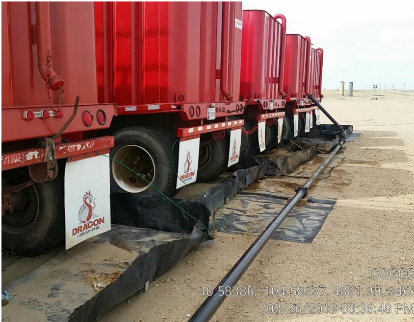
Photo 1 – Flowback Tanks have been grounded and bonded
