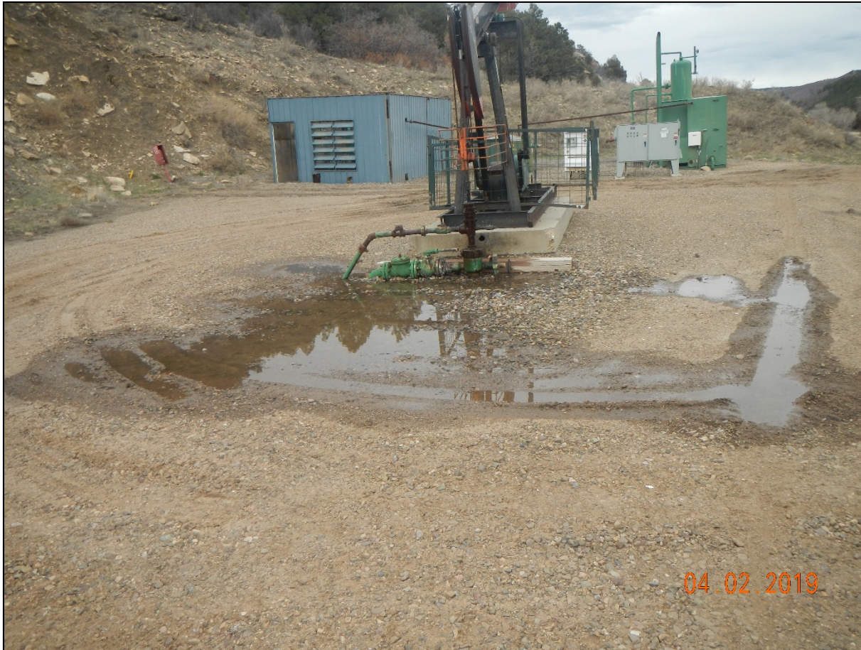
Photo 1. There is PW leaking from the wellhead.
