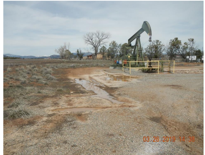
Pooled fluids and discolored soil surrounding #30-2 well head.
