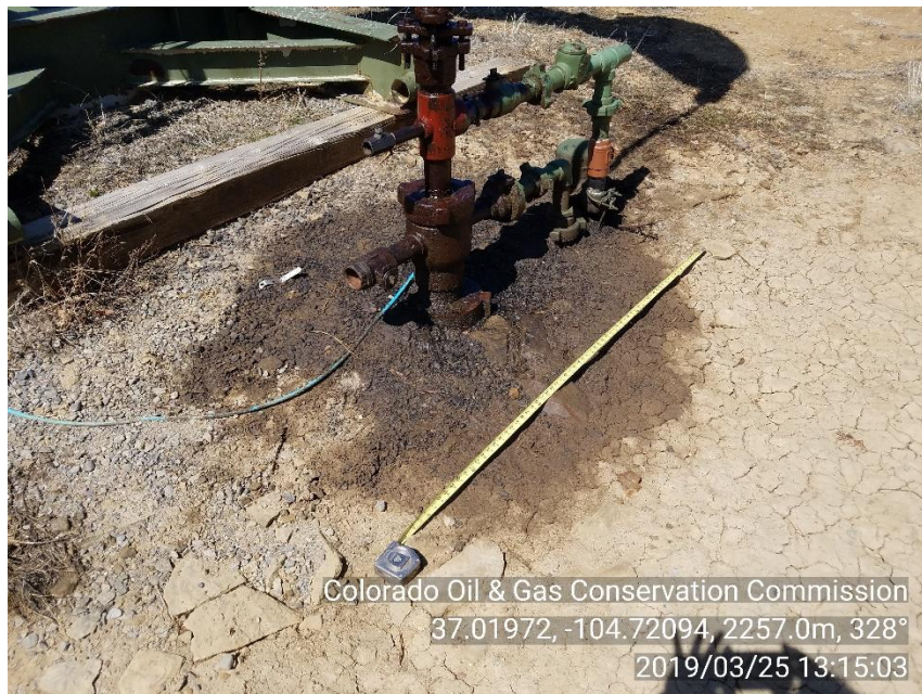
PHOTO 3: WELLHEAD IS SOAKED WITH AN OILY SUBSTANCE THAT IS IMPACTING A 5' BY 4' RADIUS AROUND WELLHEAD
