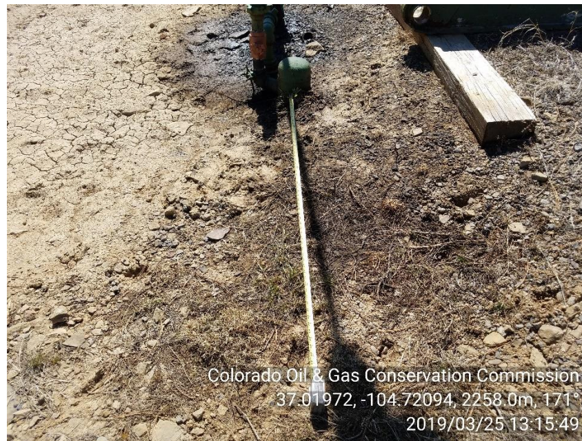
PHOTO 4: IMPACTED SOIL APP. 4' BY 3' TO THE NORTH OF WELLHEAD
