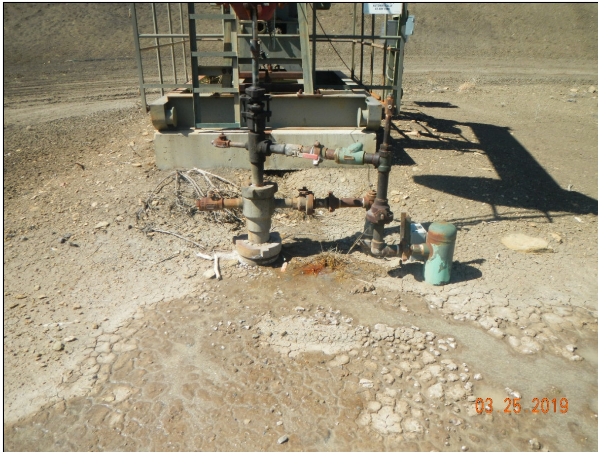
Photo 3. Water is leaking from the wellhead.
