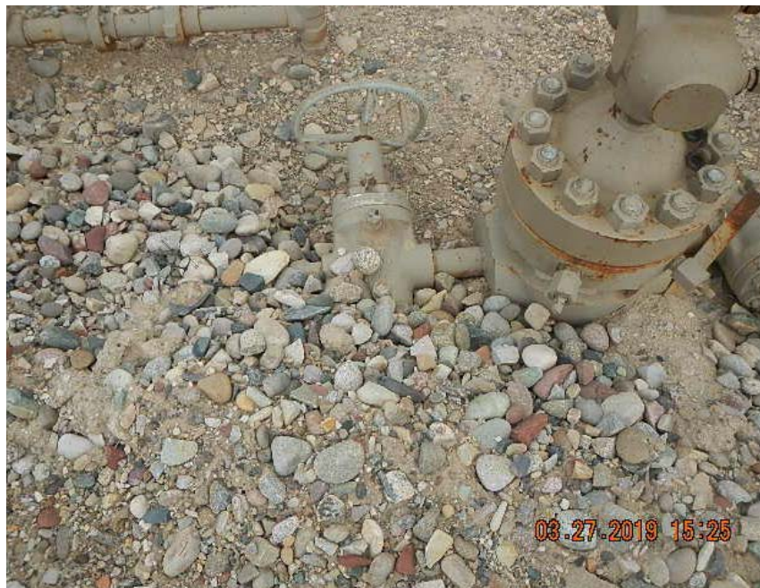
Debris has been pushed over well head equipment
