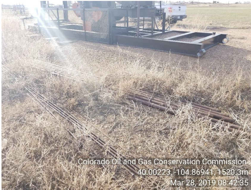
Photo 5 Unused equipment Sucker rods and tubing
