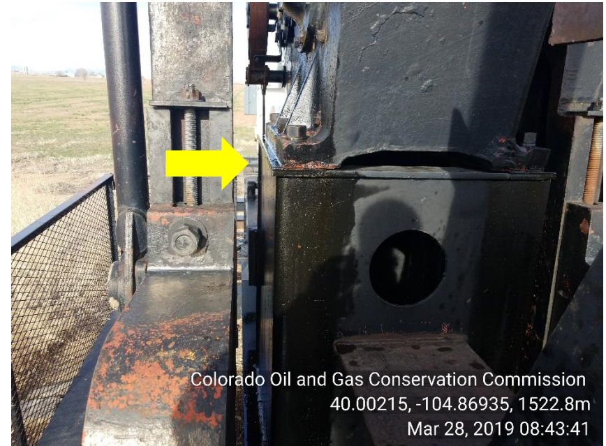
Photo 8 Mechanical issue: Gear box appears to be leaking
