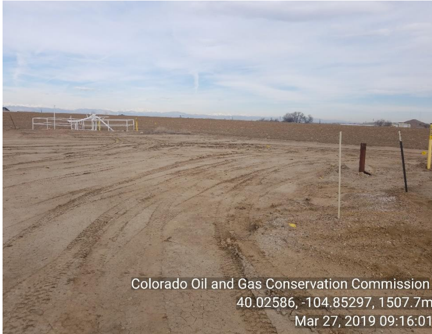
Photo 1 Well is P&A production equipment and well head are removed.
