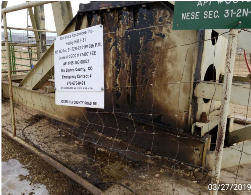
Photo 3. Oily waste on side of pump jack.
