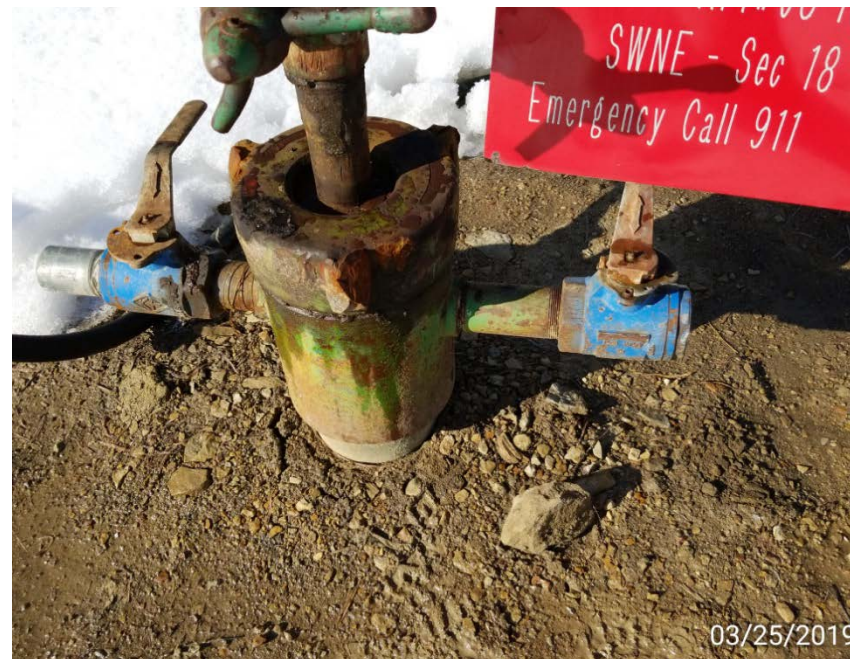
Photo 2. Gas leak on casing ball valve without pull plug.
