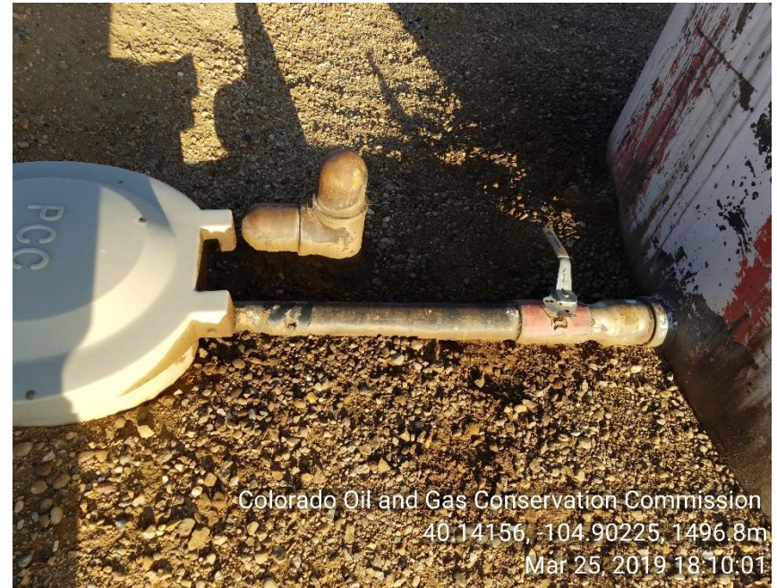
Photo 2 Stained soil under crude oil load out line
