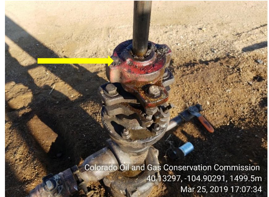
Photo 4 Mechanical issue: Fluid appears to be leaking out of packing
