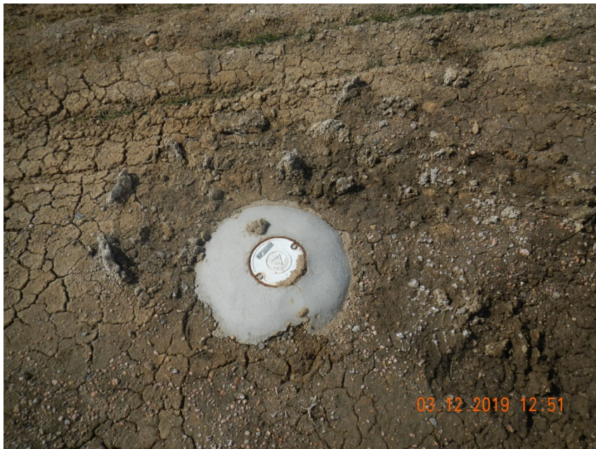
Photo 5. Photo taken from the location. Photo depicts one of the six ground water monitoring wells on location,
