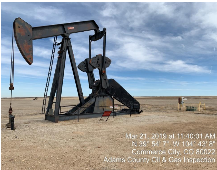
Photo#5 Wellhead/Pumpjack/Electric Motor
