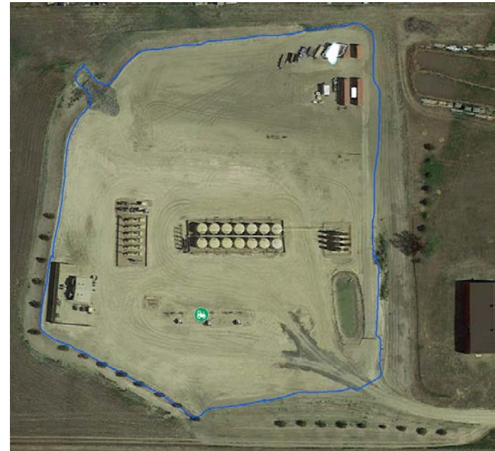
Photo 12. Aerial imagery showing the current 5.35 acre disturbance area in the blue polygon. The approved 2A stated a disturbance area of 4.8 acres during construction and 1.6 acres after interim reclamation, which should have been completed by 1/28/2018 (6 months after production of the last well on location which was 7/28/2017).
