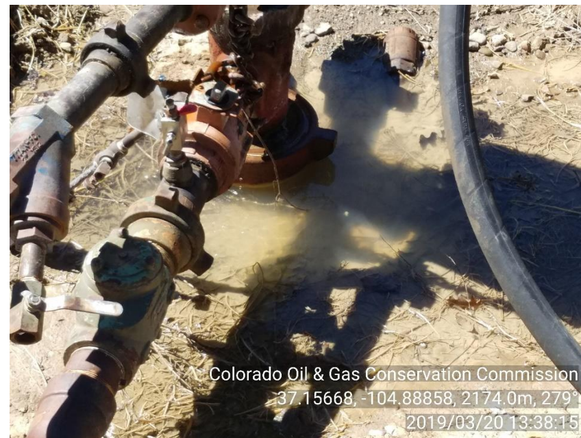
PHOTO 6: PRODUCED WATER IS POOLING INSIDE WELLHEAD CELLAR
