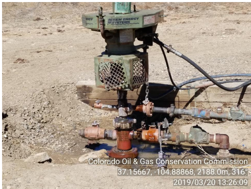
PHOTO 5: PACKING ON TBG IS LEAKING
