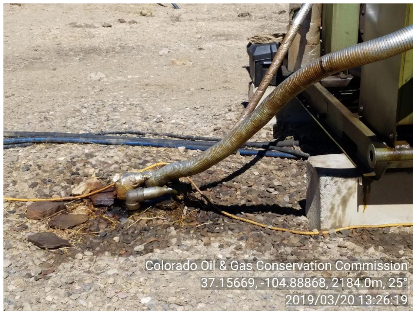
PHOTO 3: IMPACTED SOIL AROUND ENGINE SKID
